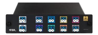
The 4FIBR CWDM solution allows the single-mode fiber to transmit up to eight 10Gbps channels. CWDM separate the data channels using multiplexer of different wavelengths into one optic thread. The 4FIBR CWDM unit is a passive Fanless unit that does not require a power source.
